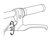
1 To adjust the brake cable play, thread the brake lever adjuster in or out 1/4 to 1/2 turn until the desired brake adjustment is attained. Most adjustments are complete at this step. If brake still needs further adjustment, proceed to step 2 for rear or step 4 for front.
