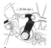
**2** If the brake has too much slack, loosen the rear anchor bolt and pull the brake wire tighter. The distance of the brake wire between the end of the cable and the anchor bolt should be between 37 and 44 mm.
