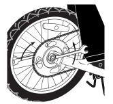
2 Loosen rear axle by attaching wrenches to both axle nuts and loosening counter-clockwise. Pull chain off sprocket and remove wheel from frame.
