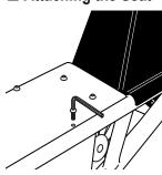
1 Remove the four bolts from the frame with the 5 mm hexagonal key wrench.
