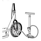
1 Using a bicycle style tire pump equipped for a Schrader-type valve, inflate the tire to the PSI indicated on the sidewall of the tire.
