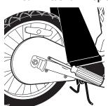
**1** Remove chain guard with Phillips Screwdriver.
