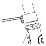
**3** Once stem is all the way down and no more threads on fork are visible, tighten two collar bolts with 5 mm hexagonal key wrench.
